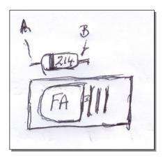
As the relay is not operated the meter should read 26v. I my case it read almost zero volts. "**relay operated**", to confirm this move probe from B to A the voltage is 26V. Switch off the cabinet allow time for voltages to leak away.
